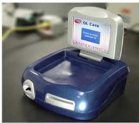
The QLCA represents a shift in the design POC analyzers. The QLCA is small, portable, stand-alone and completely automated point-of-care immunoanalyzer. The QLCA has successfully miniaturized lab test technology, and combined it with a simplified mechanical design and proprietary triggering mechanism.
