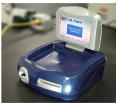
The QLCA represents a shift in the design of POC analyzers. The QLCA is a small, portable, stand-alone and completely automated point-of-care immunoassay analyzer. The QLCA has successfully miniaturized lab test technology, and combined it with a simplified mechanical design and proprietary triggering mechanism.
