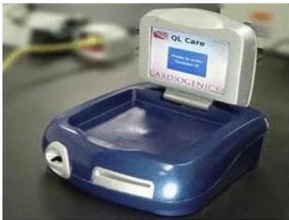
The QLCA represents a shift in the design of point-of-care (POC) analyzers. The QLCA is a small, portable, stand-alone and completely automated POC immunoassay analyzer. The QLCA has successfully miniaturized lab. test technology, and combined it with a simplified mechanical design and proprietary triggering mechanism.
