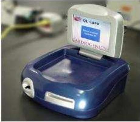
The QLCA represents a shift in the design of point-of-care (POC) analyzers. The QLCA is a small, portable, stand-alone and completely automated POC immunoassay analyzer. The QLCA has successfully miniaturized lab. test technology, and combined it with a simplified mechanical design and proprietary triggering mechanism.
